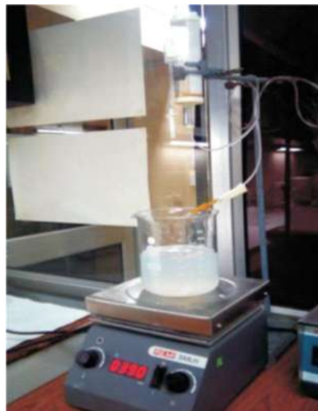
Fig.-1: Scale up synthesis of Cu-chitosan Nanoparticles.
