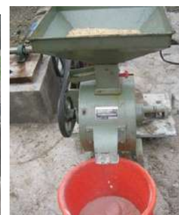
Plate-1, 2 : Using flour mill jowar flour were obtained from bullock operated power transmission system.
