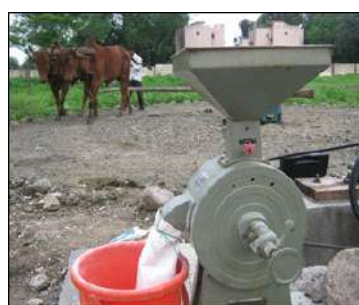
Plate-1, 2 : Using flour mill jowar flour were obtained from bullock operated power transmission system.
