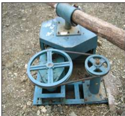
Animal driven rotary power transmission unit
