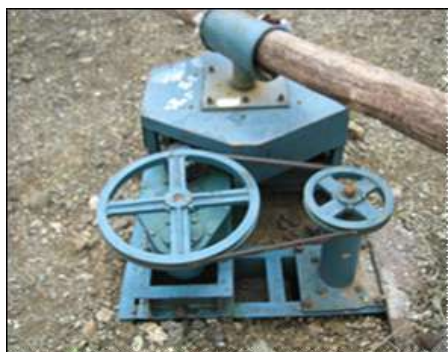
Plate No. 1. Gear box unit for mechanical power in rotary mode.
