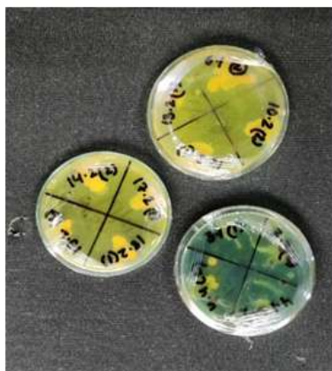
Figure : Bromo Thymol Blue (BTB) test.
