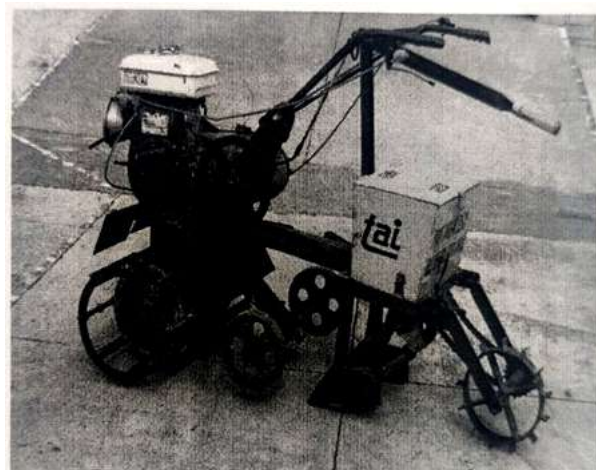
Fig-1 : Schematic view of power tiller operated seed cum fertilizer drill.
