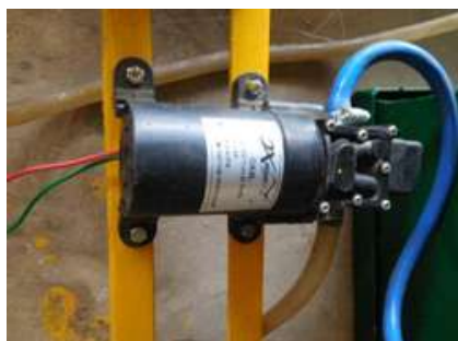
Fig.-3 : Supply pump (12 V DC) with motor.
